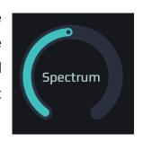
The Spectrum parameter lets you adapt the measurement to the spectral balance of your source material. Most real-life music signals approximate a so-called **pink spectrum**, where the energy towards higher frequencies decays with 3 dB per octave, which is the default and center of the spectrum parameter.
