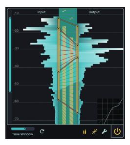
The **curve display** shows you how the adjustments you make to the handles affect the Dynamic Grading's internal gain curve. If you've grown up with compressors, this is another way for you to connect with the "old world".
