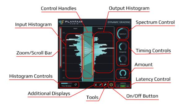
Dynamic Grading's user interface is built around the main display, which shows the dynamic histograms for the input and output signals. The area between the two graphs provides graphical control handles to intuitively adjust the dynamic processing.
