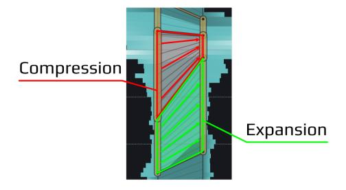
When the target range is narrower than the corresponding source range, this part of the dynamic range will be compressed. If it is wider, it corresponds to an expansion of dynamic range.
