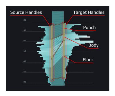
The yellow shapes in the middle between input and output histograms can be freely manipulated by dragging them around with the mouse. The handles on the left (input) side are called source handles, the ones on the right (output) target handles. We call the yellow bars "ranges", and the little dots "reference points".
