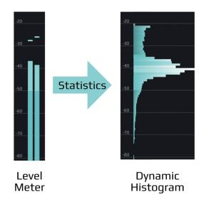
Now imagine a *really fast-moving* level meter like the one on the left, and a superhuman statistician sitting in front of it, looking up the level on the meter *really often* and keeping a tally sheet of how often she or he reads each possible value over – say – the last 20 seconds. The result is plotted as a bar graph like the one on the right. In the example above, you can see that values around -40 dB have occurred much more often than values around -50 dB or -16 dB, as an example.
